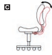
C Back angle adjustment back angle adjusts independently with a single lever.
