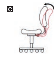
Back angle adjustment back angle adjusts independently with a single lever.
